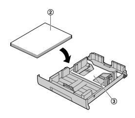
4 Adjust the recording paper guides. Pinch the front side of the recording paper guide (4), then slide it to
