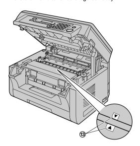
8 Close the top cover by holding the indentations on both sides of the unit, until locked.
