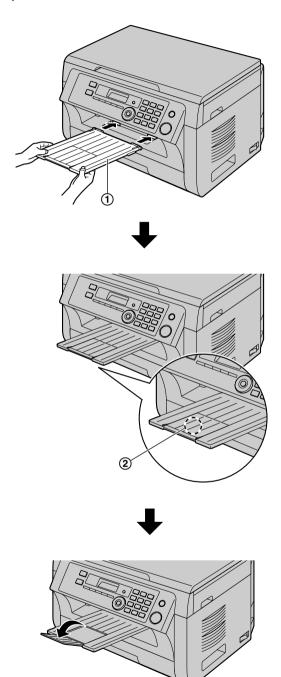
vary depending on the usage environment). Remove the printed paper before the output tray becomes full.
